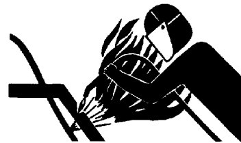
Heating Near Pressurized Fluid Lines
