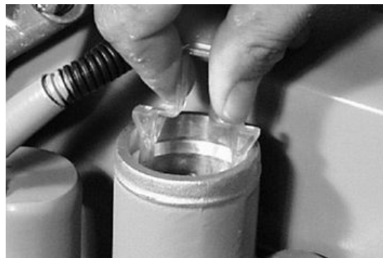
Removing Thermostat from Housing (Earlier Engine Shown)
